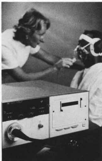
Ear Oximeter measures O 2 saturation non-invasively, continuously — independent of skin pigmentation, ear thickness, ear-piece motion. No individual patient calibration needed.
