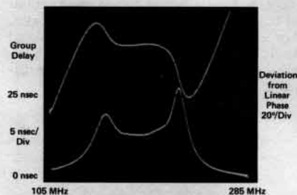
Figure 5. Two independent techniques for measuring filter phase distortion
