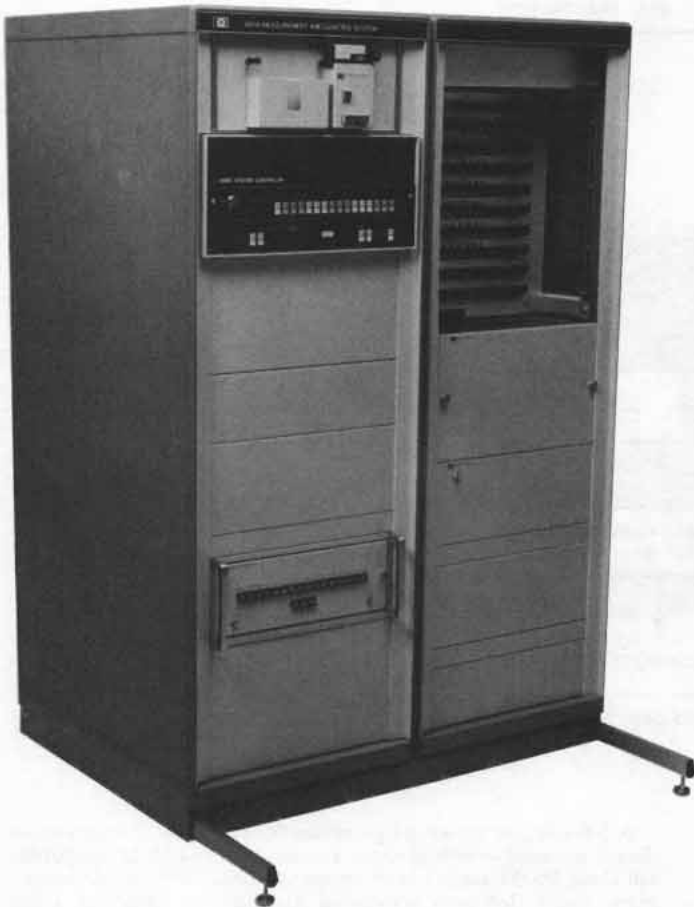
Industrial measurement and control system (doors removed to show screw-terminal signal connection assemblies).
