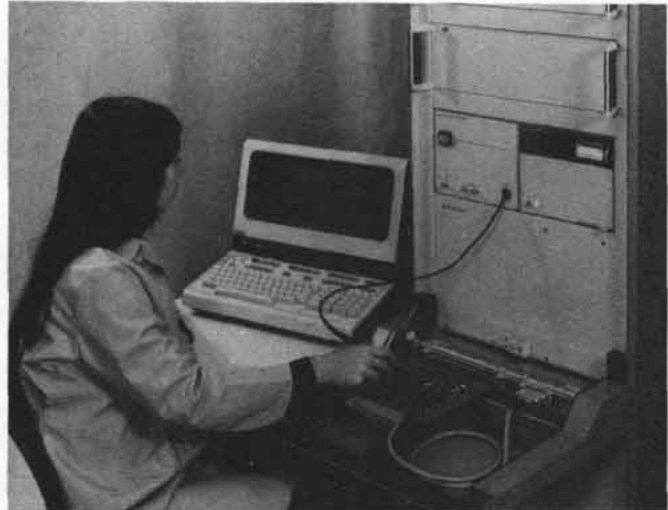
Computer-assisted guided probe fault location
